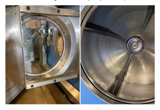
The images above show the results on the washing machine windows and internals after 5 months. The windows are no longer caked with scale and the internals remain
