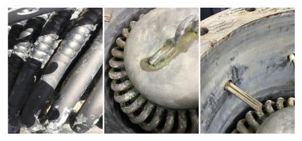
The images above show the heater core after 3 months of the trial. Following the trial no removal for cleaning was necessary, only visual inspection and re-sealing.
