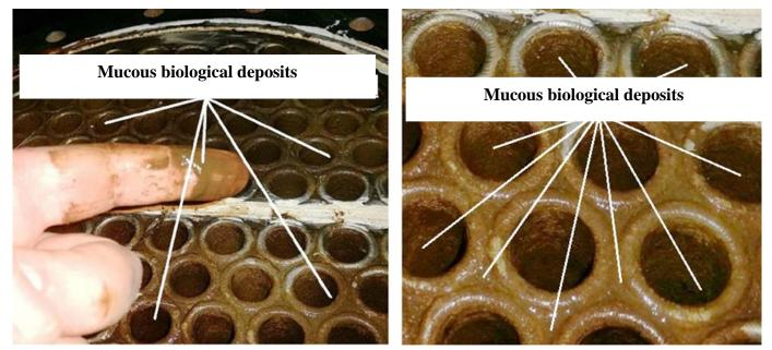
Mucous biological deposits on the tube plate at the beginning of the test installation
