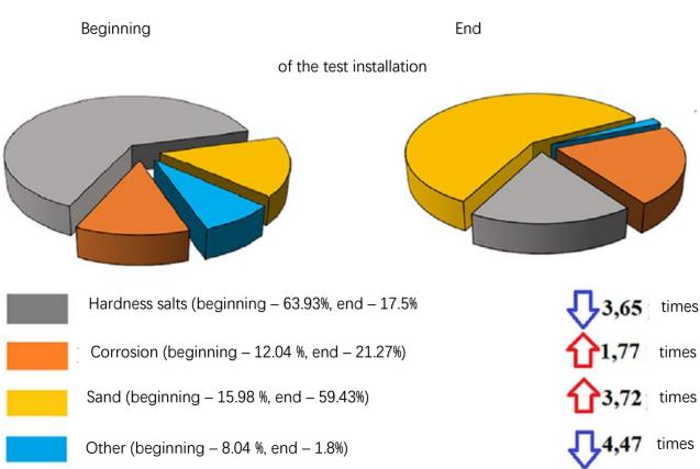
Changes in the structure and chemical composition of deposits on the inner surface of the industrial water supply pipe
