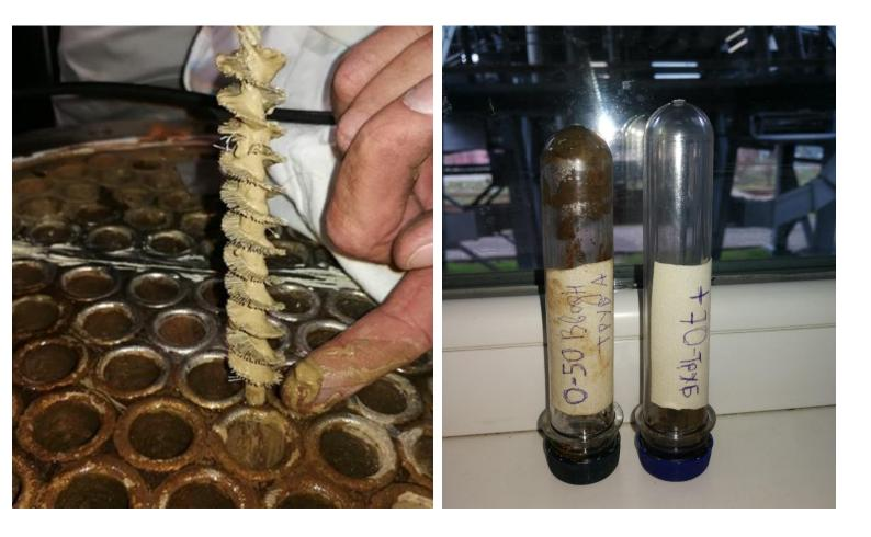
Sampling deposits from the inner surface of the wall of the heat transfer tube
